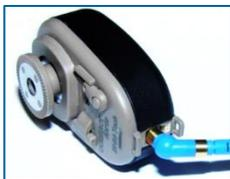
The programming socket on the **contact forte** is located at the bottom of the hearing system and is protected by a socket cover and a socket seal that must be removed before the programming cable is connected.
