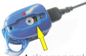
4-pin programming socket
