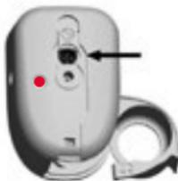
**i** Please ensure that the red marking on the programming cable plug is on the same side as the yellow marking on the programming socket. Otherwise, you will have no connection or may destroy the programming socket!
